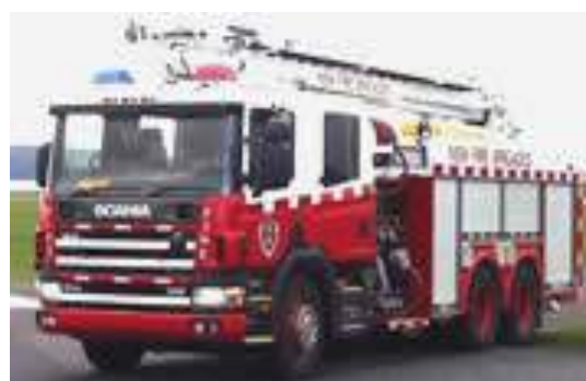
Aerial pumper: 20 tonnes (Gross Vehicle Mass)
