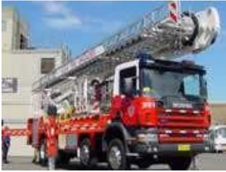
Ladder platform: 26 tonnes (Gross Vehicle Mass)
