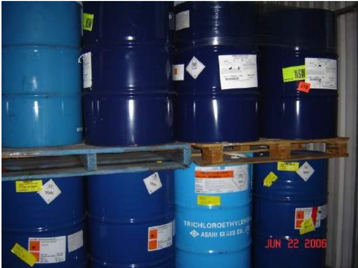
Chemical drums showing safety placards, which must be quickly identified.
