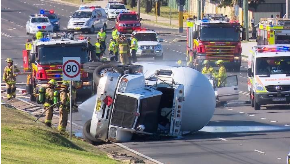
Dangerous goods signage on can be seen on the overturned tanker (red diamond near the number plate).
