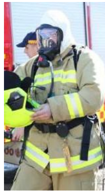
The self-contained breathing apparatus mask sits over the mouth, resulting in decreased voice projection and muffled speech.
