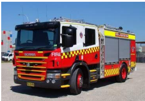
Urban pumping appliance: 15 tonnes (Gross Vehicle Mass)
