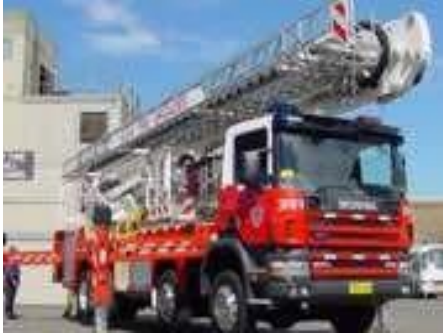
Ladder platform: 26 tonnes (Gross Vehicle Mass)
