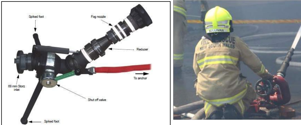
Figure 9 A firefighting monitor
