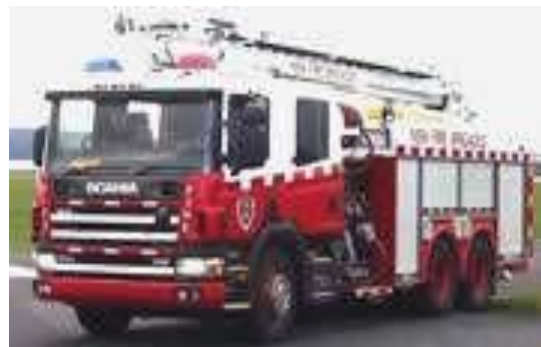
Aerial pumper: 20 tonnes (Gross Vehicle Mass)
