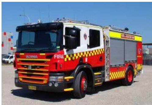
Urban pumping appliance: 15 tonnes (Gross Vehicle Mass)
